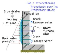
HYDROPROOF WP-GS Adhesion Ground granul urnace slage for
