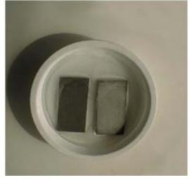
200th freeze dissolution and the 250th time. Underwater freeze state. The circumference is deleted considerably and the unsettled concrete version can check a small hole on the surface.
