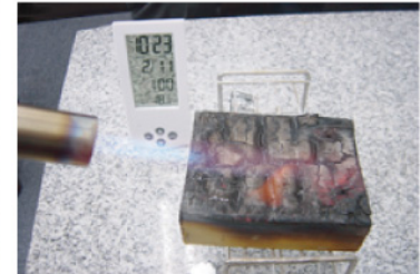
The core is showing high temperature. Gradually put the fire away from the wooden chip, but it doesn't start to burn itself.
