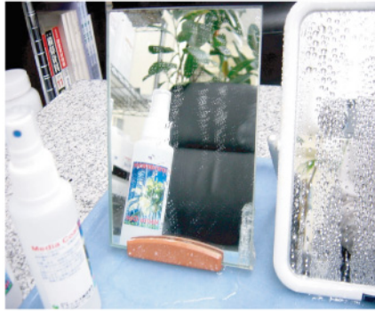
Un-processed mirror remains many water drops on its surface.
