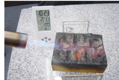
The core is showing high temperature. Gradually put the fire away from the wooden chip, but it doesn't start to burn itself.
