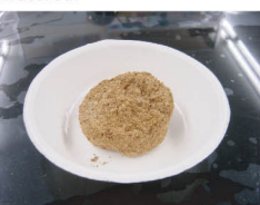
Completely dried (for one year) wooden piece to which G-1+G-2 is applied: Water-retention effect appears again when the piece is watered.
